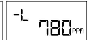
3. Please see Fig. 3 for LCD screen display. Fig. 3-a is LCD display in normal operation state, while fig. 3-b is LCD display in the state of relay control point setting.
