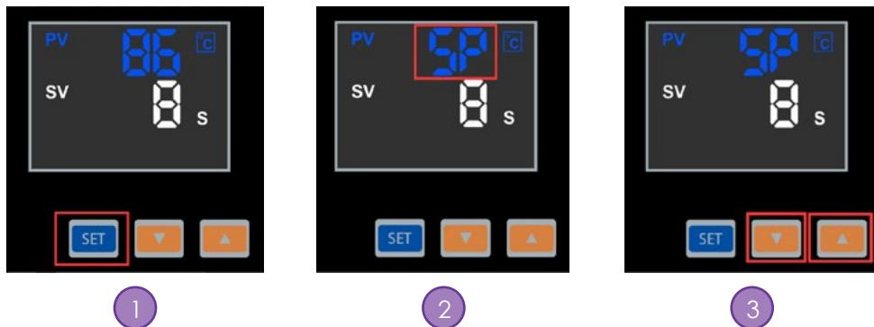
Press once again the "SET" button, on the screen the "St" will show up. Press "▼" or "▲" for the desired time.
